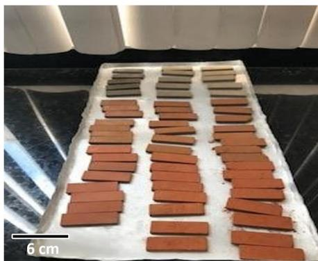
**Figure 1.** Raw and fired specimens
